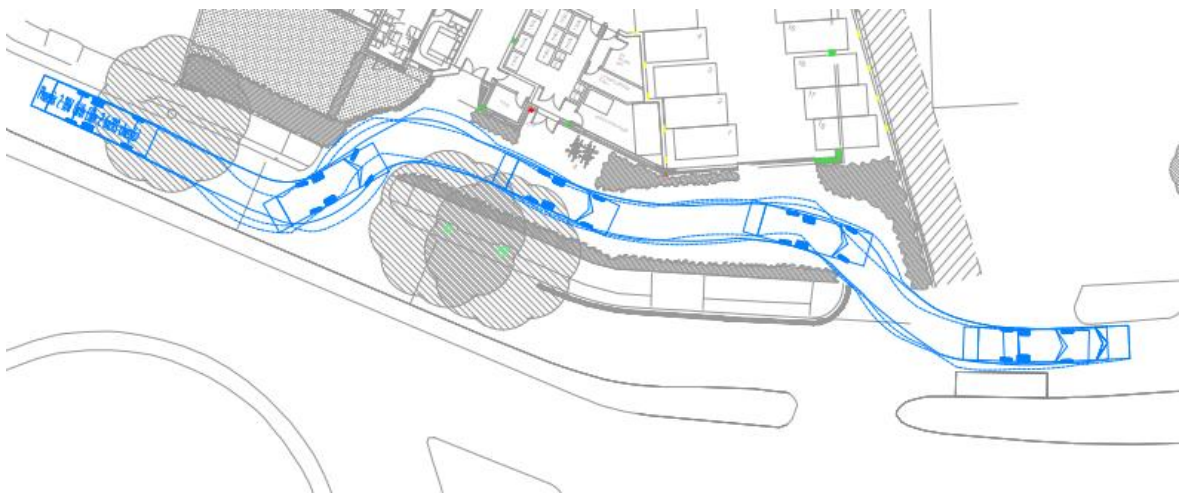
Figure 1: Refuse Vehicle Swept Path
