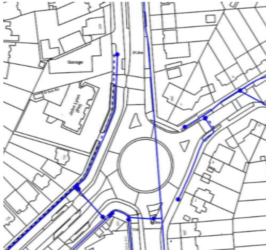
Figure 3: Existing Water Mains
